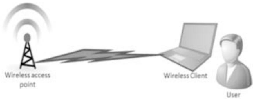
Figure 1. Wireless networking components.
